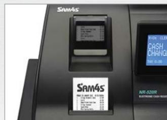
• Single & Twin Station Thermal Printers.
