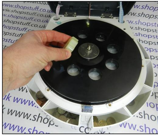
3. Brush metal sorting disk and gently vacuum foam underside of plastic disk, checking for holes or damage to the underside of the disc at the same time.
