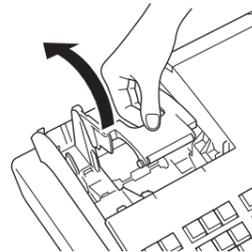
2. Ensuring the paper is being fed from the bottom of the roll, lower the roll into the space behind the printer.
