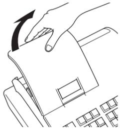
2. Remove the battery compartment cover.
