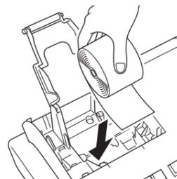
3. Put the leading end of the paper over the printer.
