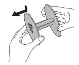
**3** Slide the leading end of the paper into the groove on the spindle of the take-up reel and wind it onto the reel two or three turns.
